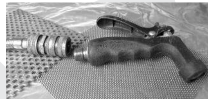
Hot and cold water can be hooked up with readily available (and inexpensive) garden hose disconnects.
