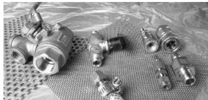
Left, NPT threaded plumbing fittings, not quick; center, Swagelok® tubing fittings, sort of quick; right, quick disconnects, expensive and hard to clean.
