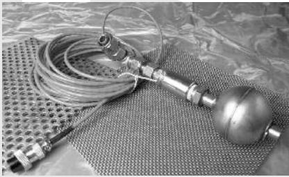
Float switch connects to the grant, turns on pump when level rises.
